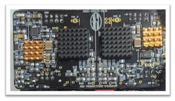
Thanks to a world-class PCB design, a refined selection of top-quality audio grade components, and the extremely efficient GaN-based power stage we achieved the design's goal to operate this integrated Stereo Version of at >600kHz as main PWM frequency. The higher PWM frequency operation delivers a direct and positive impact on the overall outstanding sonic and musical performances with sublime mid-high range realism along with the unique tight and controlled bass register.
