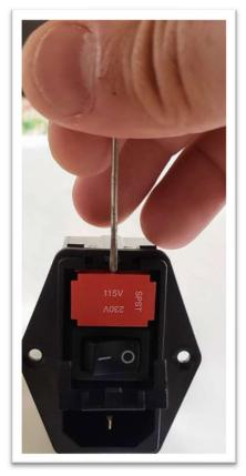
The voltage selector block also contains the fuse holder and it is accessible by opening the plastic cover that holds it within the IEC power entry module, as shown in the following picture.
