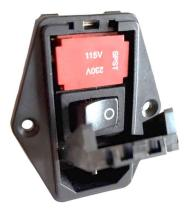
The Voltage selection is done by extracting the voltage selector block and re-inserting it with the voltage label readable (not up-side down) and then closing the plastic door.
