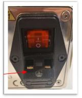
The AGD "ALTO MKII" has a universal voltage input configuration and can operate between  $90^264VAC\ 50/60Hz\ single\ phase$ .
